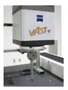
VAST XT probe head combines the two probing technology: point-to-point measurement and high-speed scanning measurement. This enables dimension measurement as well as profile inspections and position inspections.
