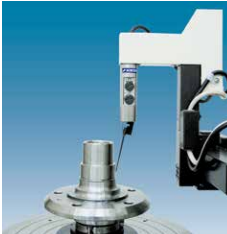
Sample roundness measurement of outside diameter
