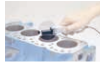
Nose Piece (For Flat Surfaces) E-WJ-S88A For handheld measuring of a flat surface whose measuring surface is too small.
