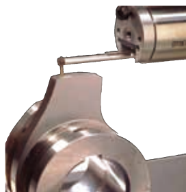
Sample skidless measurement
