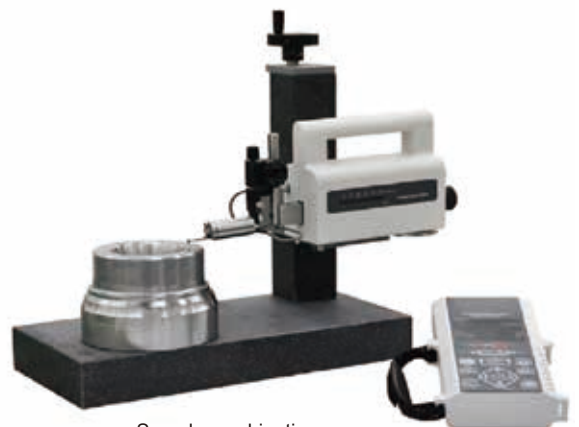
Sample combination with a compact measuring stand (option).
