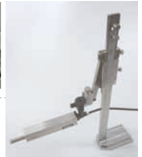
Sample combination of a tracing driver and height gage
