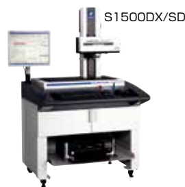
Specialized machine for roughness measurement
