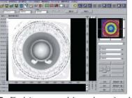
Profile dot sequence data can be captured using PS200 Profile Scanner or 3000A-3DF SURFCOM as a digitizer.
