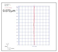
Up/down direction verticality (using straight edge)
