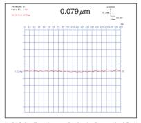
Left/right direction verticality (using optical flat)
