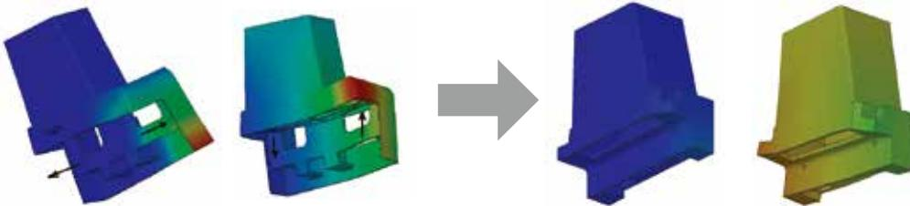
The ideal right Y-column design (modularized components, lightweight, improved rigidity) obtained using CAE provides SVA series machines with higher speed characteristic and lower repeatability error for high speed and high accuracy. Compared with previous models, the SVA-A measuring machine provides 1.5 times more rigidity overall.
