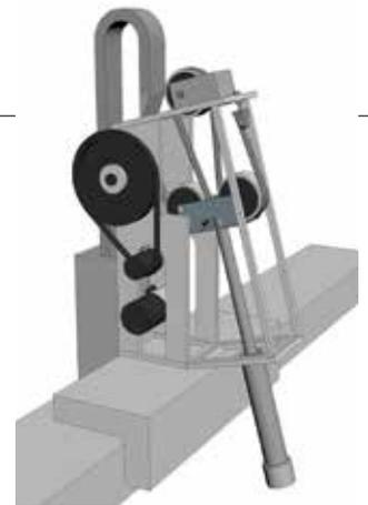
Image of Z-axis motor configuration
