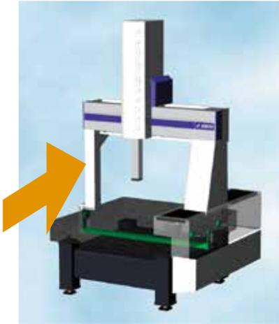
The Y-axis guide surface generally has a second guide surface (sub-guide) on the right side of the table. The maisonette bridge structure provides guide surfaces on both sides of the table, which eliminates the chance of variations in sub-guide connectors (screws, adhesives, etc.) over time. This simplifies the structure, which improves rigidity and simplifies guide plate processes for higher accuracy.
