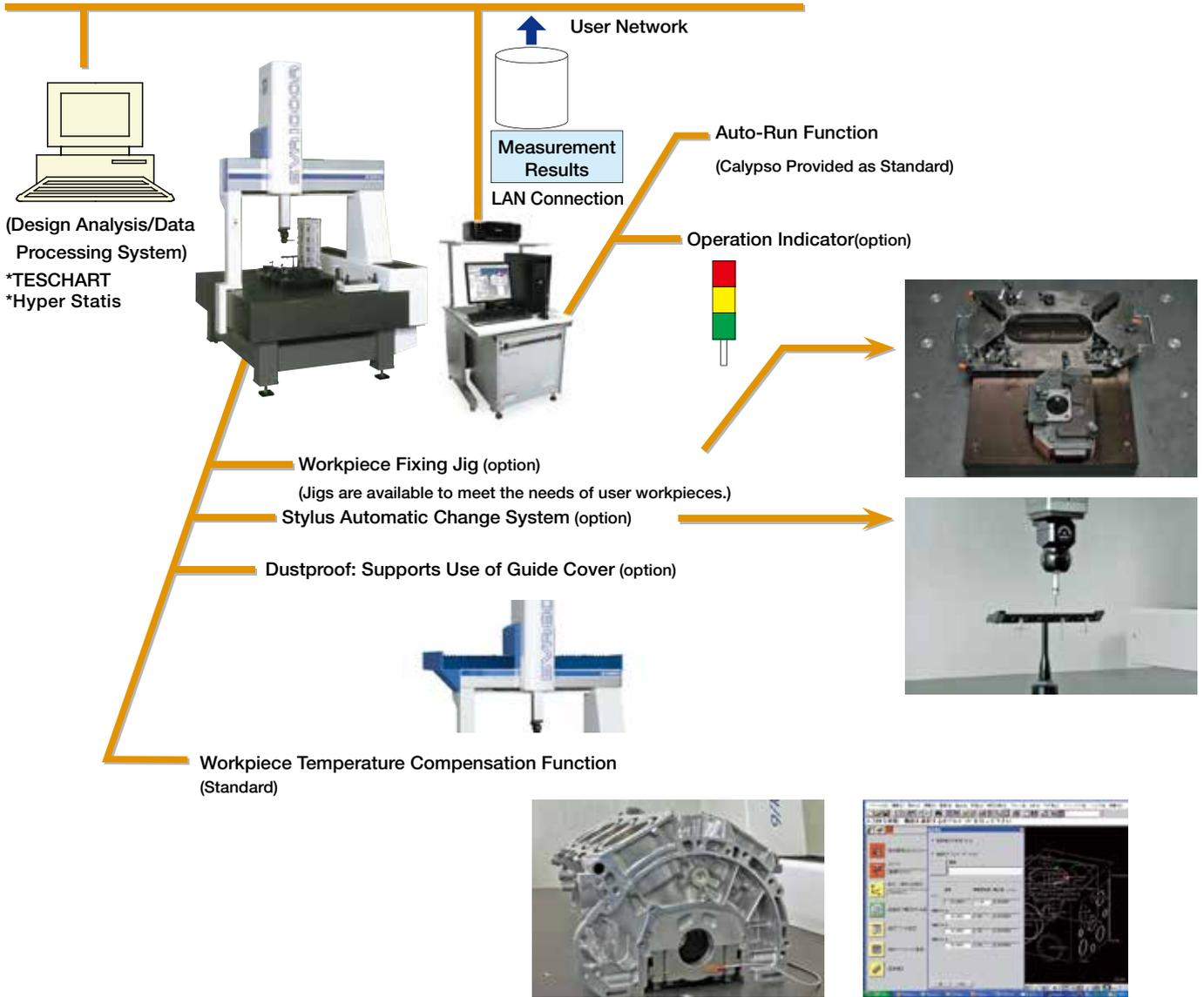
The measuring machine and workpiece temperatures are controlled in accordance with the measuring environment's influence on the measuring machine.
