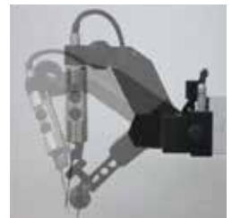
Example of effective workpiece measurement with the offset type detector holder
