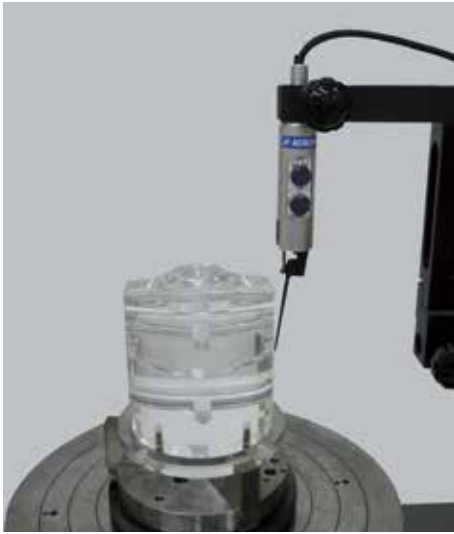
Sample roundness measurement of outside diameter
