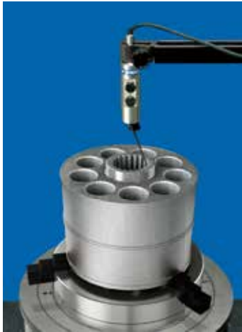
Example of roundness measurement of uncontinuous inner diameter surface
