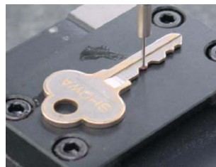
Sample measurement with PRISMO Scanning measurement of 1.0 mm thick key with 0.6 mm diameter probe (Scanning of unknown profile)
