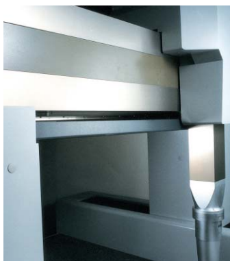
CARAT guides keep influence due to ambient temperature changes to the absolute minimum.
