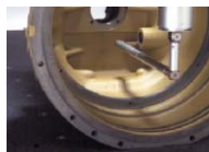
Combination probe (600mm overall length)
